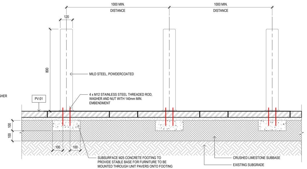
PROPRIETARY BIKE RACKS ON UNIT PAVING FN06
