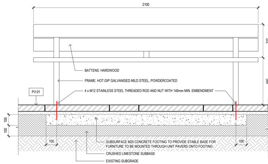
**PROPRIETARY SEAT ON UNIT PAVING FN01**
