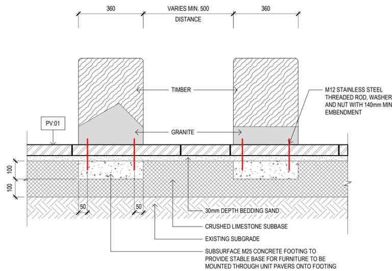
PROPRIETARY BLOCK SEAT ON UNIT PAVING FN04
