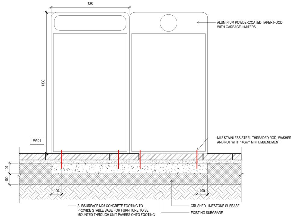
PROPRIETARY BIN ENCLOSURE ON UNIT PAVING FN05
