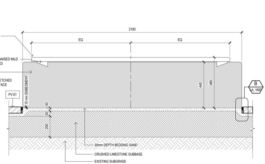
PROPRIETARY BENCH ON CONCRETE BLOCK FN03
