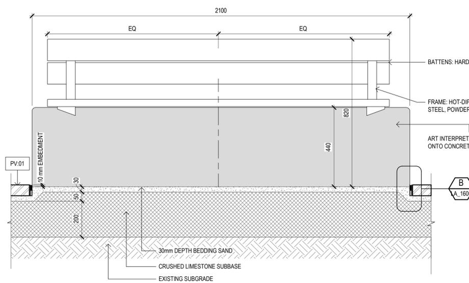
PROPRIETARY SEAT ON CONCRETE BLOCK FN02
