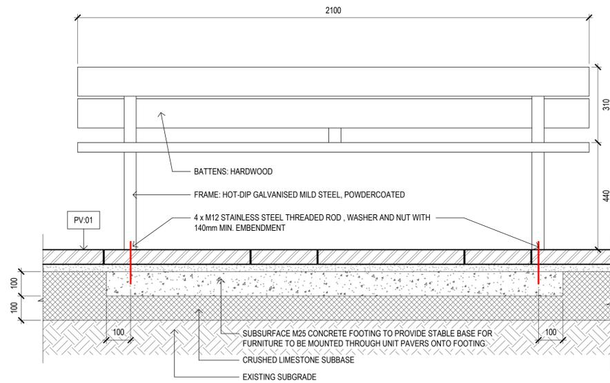
PROPRIETARY SEAT ON UNIT PAVING FN01
